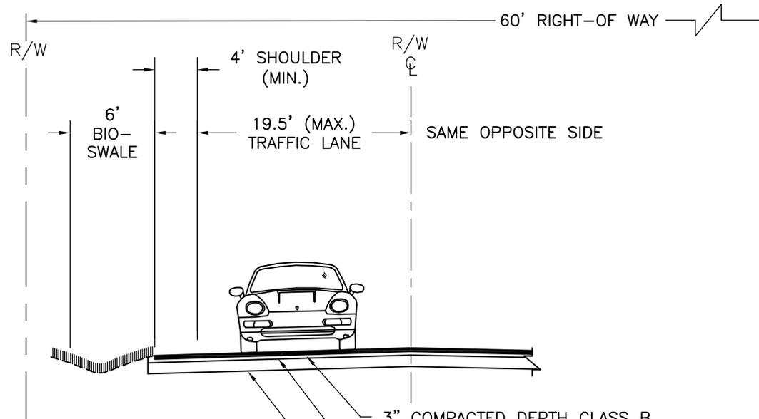
3" COMPACTED DEPTH CLASS B ASPHALT CONCRETE
