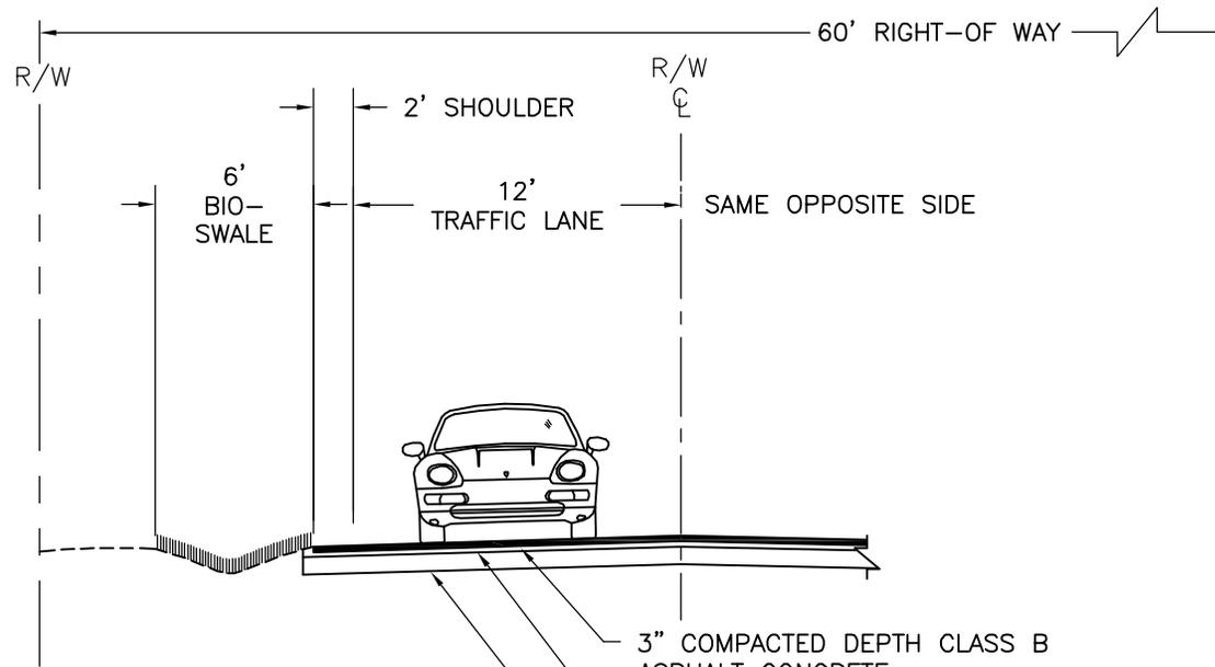
3" COMPACTED DEPTH CLASS B ASPHALT CONCRETE
